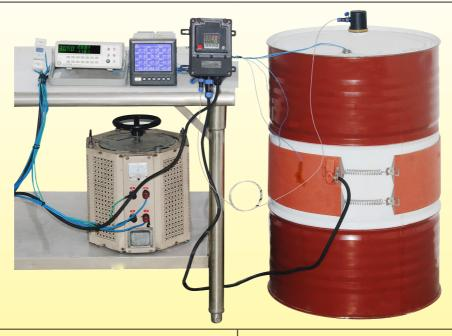
Variation in the temperature versus time of a 220-liter metal drum, filled with water, heated by a silicone heating belt 200mm wide, without thermal insulation, power 2250W (surface load 0.75W/cm²).
